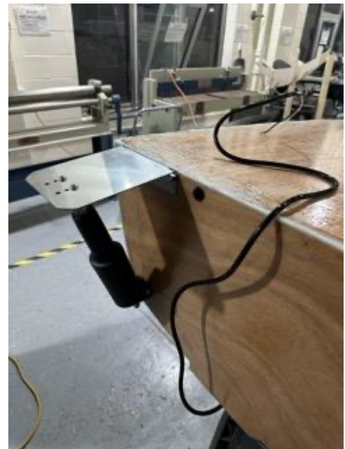
Figure 5: Trim tab for steering control
